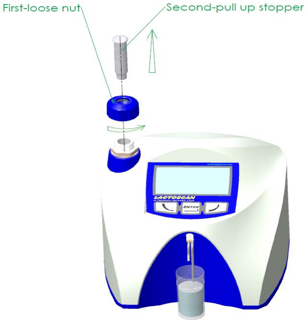
Fig. 7 Placing the stopper
